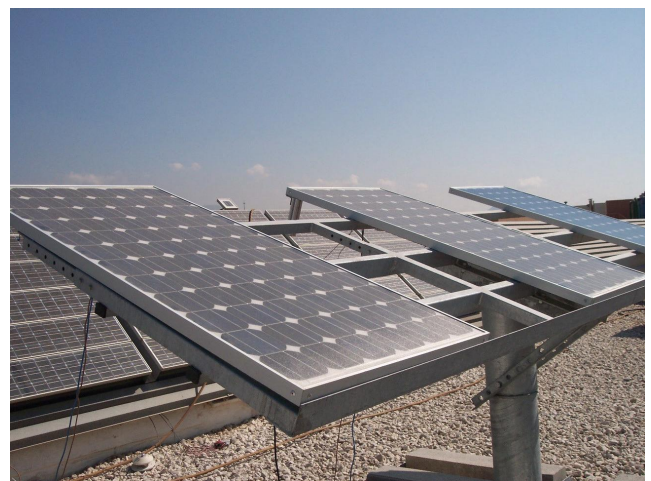
Fig. 4: Facility set-up for monitoring outdoor performance of structured glass modules compared to flat surface modules.
